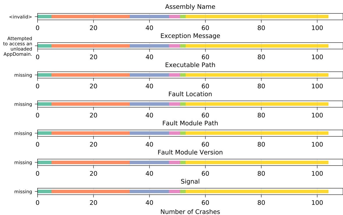
Figure 3.6: All other crash properties of the crashes with the System.AppDomainUnloadedException for the tuple ( |clr, fullclr, 2.0.50727| ) in Figure 3.5b .
