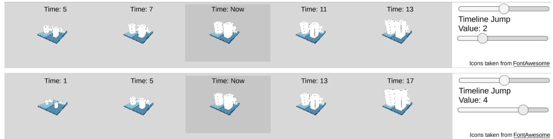
Figure 17: This image demonstrates the synchronized timeline view when the timeline jump value has been altered. On the top the timeline jump value is two and on the bottom its four.
