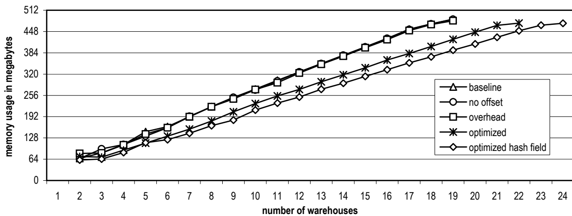
Figure 5.12: SPECjbb2005 laptop: average used memory after a full garbage collection (lower is better)
