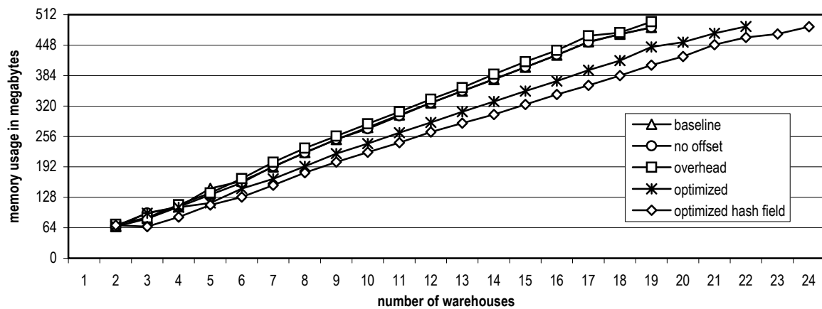
Figure 5.6: SPECjbb2005 laptop: average used memory after a full garbage collection (lower is better)
